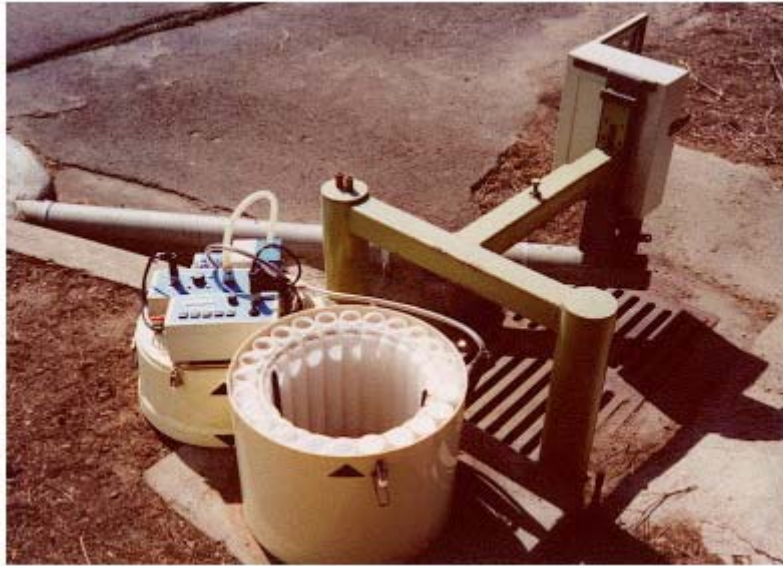
Figure 3. Gamet grab sampler showing sample bottles.
